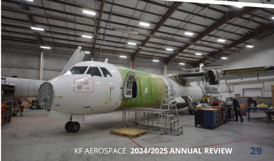
An ATR72-500F undergoes a cargo conversion.
